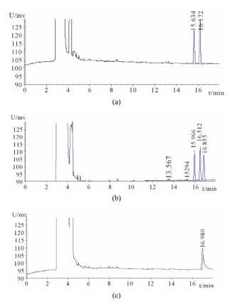
Figure 3. The GC illustration of borneol in inhalant. ((a) standard solution; (b) sample solution; (c) negative sample solution without borneol).
