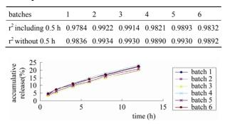
Figure 5. The dissolution release profile of borneol from inhalants in 12 hours without 0.5 hour point.
