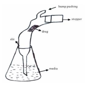
Figure 2. the test apparatus of the *in vitro* release for inhalants.
