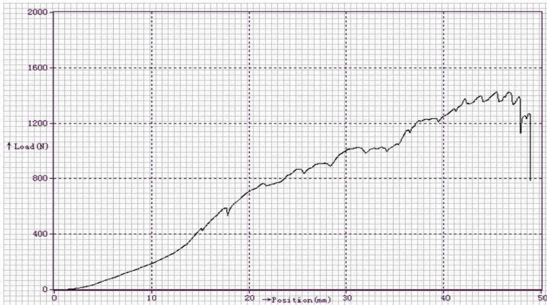
Fig. 14. Bending load-position curve for Roof Rail honeycomb
