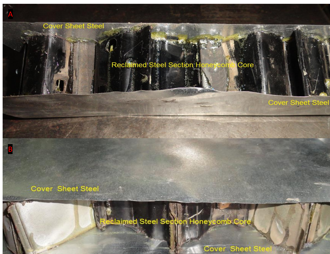
Fig. 9. Reclaimed steel sections cores are alignment between covers of Galvanized sheet steel of (0.2 mm) thickness
