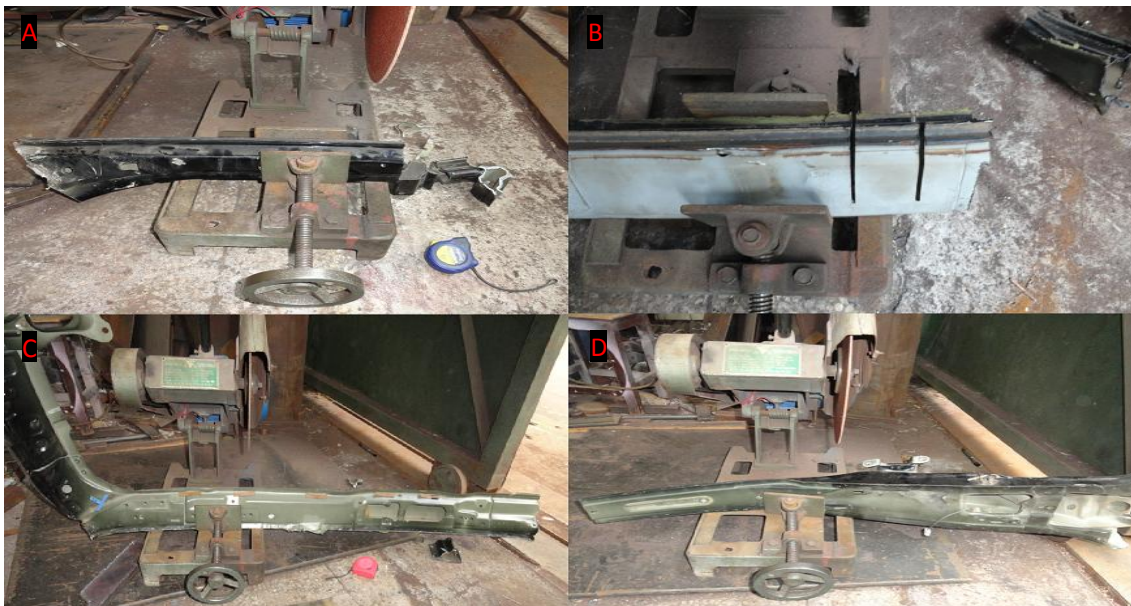
Fig. 6. Front Pillar (A), Roof Rail (B,C), and Center Pillar (D) disassembly by shearing to separate cells to be used for honeycomb sandwich preparation
