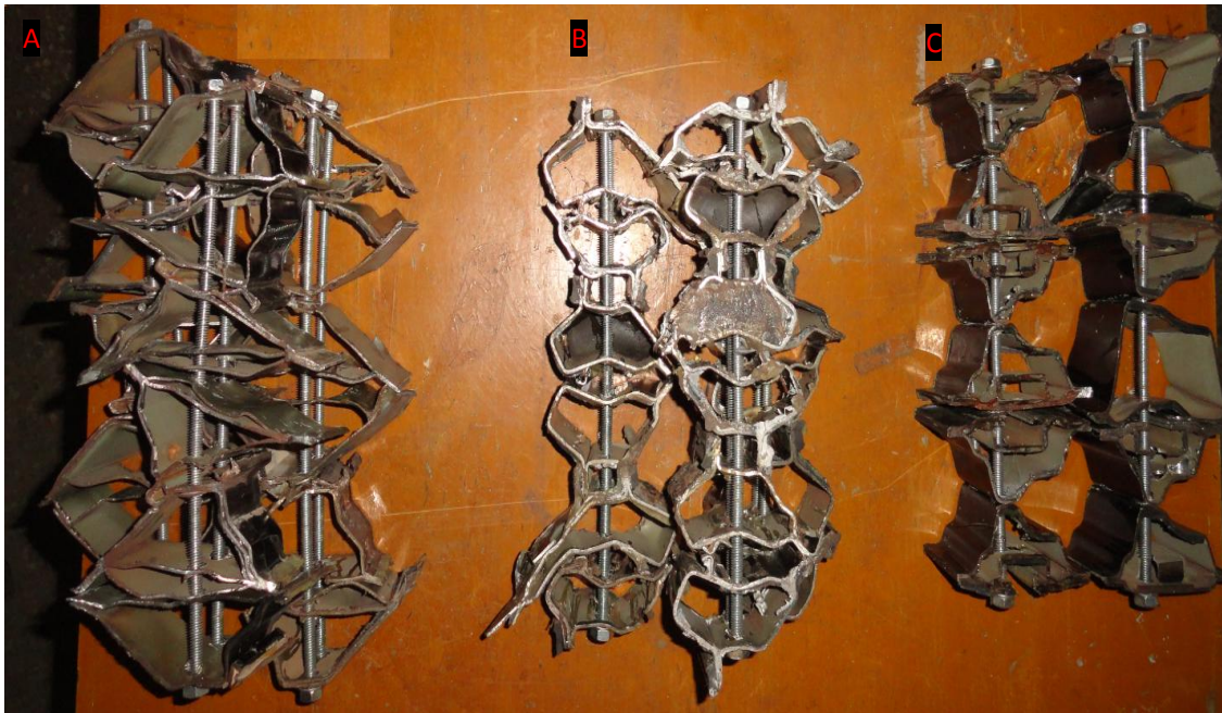
Fig. 8. Six Sheared Sections are assembly by using screws of M8 size and holes A (Roof Rail Section), B (Front Pillar Section), C (Center Pillar Section)
