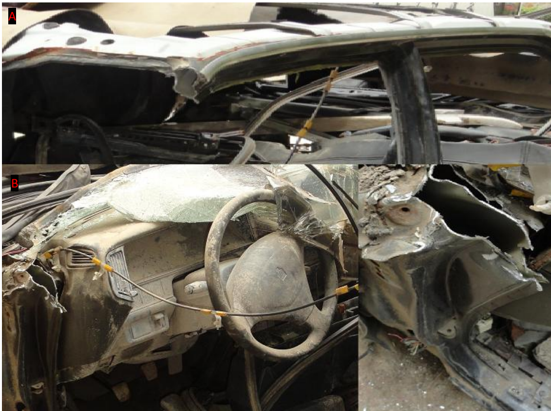
Fig. 5. End-of-life vehicle disassembly by shearing to separate several sections to be used for honeycomb sandwich preparation A (Center Pillar Section and Roof Rail Section), B (Front Pillar Section)
