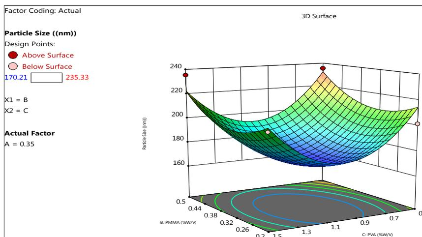
**Fig. 4. 3 D Surface Graph of Particle Size (PMMA and PVA)**
