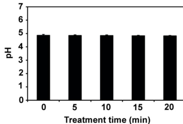
**Figure 6.** The pH measurement in the PDB media post plasma treatment of the fungal spores for 5, 10, 15, and 20 min. Untreated (0 min) fungal spores were used as a control. The pH was measured immediately after plasma treatment. Each value is indicated as the mean and standard deviation of 9 replicate measurements.
