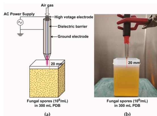
**Figure 1.** Non-thermal atmospheric pressure plasma jet device. (a) Schematic view of the plasma jet device and the experimental set-up for fungal spore treatment with plasma. (b) Photograph of treatment of the fungal spore suspension with the plasma jet.
