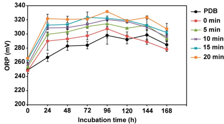
**Figure 5.** Oxidation reduction potential (ORP) measurements in the PDB media post plasma treatment for 5, 10, 15, and 20 min, or without treatment (0 min). Post plasma treatment, the fungal spores in the PDB solution were cultured for 168 h, and the ORP was measured every 24 h. Each value is indicated as the mean and standard deviation of 9 replicate measurements.
